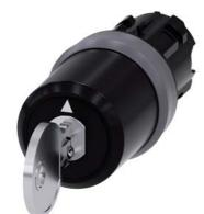
Key-operated switch BKS, 22 mm, round, plastic with metal front ring, Lock No. E2 (VW), without key, 3 switch positions I-O-II, latching, actuating angle 2x45°, 10:30h/12h/13:30h, Key removal I+O+II
