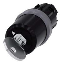
key-operated switch Siemens, 22 mm, round, plastic with metal front ring, lock no. LSG1, with 2 keys, 2 switch positions O-I, latching, actuating angle 90°, 10:30h/13:30h, key removal O+I, with laser labeling, inscription or symbol customer-specific selection with SIRIUS ACT configurator (CIN)
