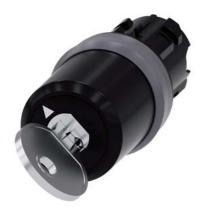
key-operated switch Siemens, 22 mm, round, plastic with metal front ring, special lock, with 2 keys, 2 switch positions O-I, latching, actuating angle  $90^\circ,\,10:\!30h/13:\!30h,$  key removal O+I
