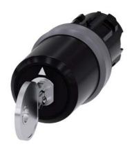
key-operated switch Siemens, 22 mm, round, plastic with metal front ring, lock number SSG10, with 2 keys, 3 switch positions I-O-II, latching, actuating angle 2x45°, 10:30h/12h/13:30h, key removal I+O+II, with laser labeling, inscription or symbol customer-specific selection with SIRIUS ACT configurator (CIN)
