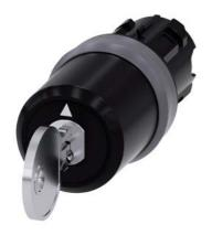
Key-operated switch BKS, 22 mm, round, plastic with metal front ring, lock number S1, with 2 keys, 3 switch positions I-O-II, latching, actuating angle  $2x45^{\circ}$ , 10:30h/12h/13:30h, key removal I, with laser labeling, upper case
