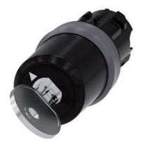
Key-operated switch BKS, 22 mm, round, plastic with metal front ring, Lock No. E2 (VW), without key, 2 switch positions O-I, latching, actuating angle  $90^\circ, 10:30h/13:30h$ , key removal O, with laser labeling, inscription or symbol Customer-specific selection with SIRIUS ACT configurator (CIN)
