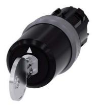
Key-operated switch BKS, 22 mm, round, plastic with metal front ring, lock number S1, with 2 keys, 3 switch positions I-O-II, latching, actuating angle  $2x45^{\circ}$ , 10:30h/12h/13:30h, Key removal I+II, Z=50-unit packaging
