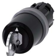
Key-operated switch IKON, 22 mm, round, plastic with metal front ring, lock number 360012K1, with 2 keys, 3 switch positions I-O-II, latching, actuating angle 2x45°, 10:30h/12h/13:30h, key removal O, with laser labeling, upper case and lower case, always upper case at beginning of line
