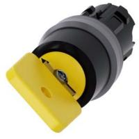
Key-operated switch O.M.R, 22 mm, round, plastic with metal front ring, lock number 73033, yellow, with 2 keys, 2 switch positions O-I, latching, actuating angle 90°, 10:30h/13:30h, key removal O, with laser labeling, lower case
