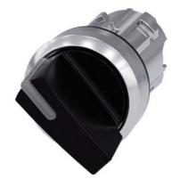
Illuminable selector switch, 22 mm, round, metal shiny, black, Selector switch short, 2 switch positions O<I, momentary contact type, Actuating angle  $45^\circ$ , 10:30h/12h
