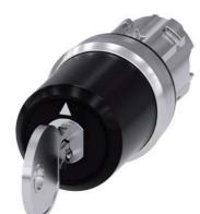
key-operated switch Siemens, 22 mm, round, metal, shiny, special lock, with 2 keys, 3 switch positions I>O<II, momentary contact on the left, latching on the right, actuating angle 2x45°, 10:30h/12h/13:30h, key removal O+II
