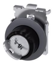
RONIS key-operated switch, 30 mm, round, Metal, matte, front ring for flush installation, special lock, with 2 keys, 2 switch positions O-I, latching, actuating angle 90°, 10:30h/13:30h, key removal O+I, possible special locks: SB31, 421, 455
