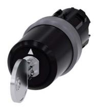
Key-operated switch BKS, 22 mm, round, plastic with metal front ring, lock number S1, with 2 keys, 3 switch positions I-O-II, latching, actuating angle 2x45°, 10:30h/12h/13:30h, Key removal II, with laser labeling, upper case and lower case, always upper case at beginning of line
