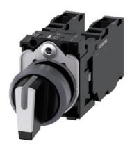
Selector switch, illuminable, 22 mm, round, plastic with metal front ring, white, selector switch, short, 3 switch positions I>O<II, momentary contact type, actuating angle 2x45°, 10:30h/12h/13:30h, with holder, 1 NO+1 NC, 1 NO+1 NC, screw terminal, with laser labeling, upper case
