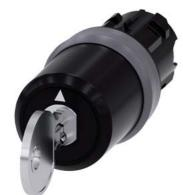
key-operated switch Siemens, 22 mm, round, plastic with metal front ring, special lock, with 2 keys, 3 switch positions I-O-II, latching, actuating angle 2x45°, 10:30h/12h/13:30h, key removal I
