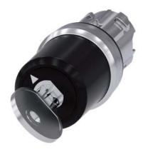
Key-operated switch BKS, 22 mm, round, metal, shiny, lock number S1, with 2 keys, 2 switch positions O-I, latching, actuating angle 90°, 10:30h/13:30h, key removal O, with laser labeling, lower case
