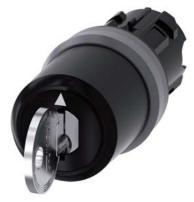
Key-operated switch IKON, 22 mm, round, plastic with metal front ring, lock number 360012K1, with 2 keys, 3 switch positions I-O-II, latching, actuating angle 2x45°, 10:30h/12h/13:30h, key removal O, Z=50-unit packaging
