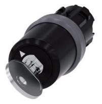
Key-operated switch BKS, 22 mm, round, plastic with metal front ring, lock number S1, with 2 keys, 2 switch positions O-I, latching, actuating angle  $90^\circ, 10:\!30h/13:\!30h,$  key removal O, Z=50-unit packaging
