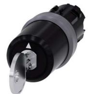
key-operated switch Siemens, 22 mm, round, plastic with metal front ring, lock number SSG10, with 2 keys, 3 switch positions I-O<II, left latching, momentary contact type on the right, actuating angle  $2x45^{\circ}$ , 10:30h/12h/13:30h, key removal I, with laser labeling, inscription or symbol customer-specific selection with SIRIUS ACT configurator (CIN)
