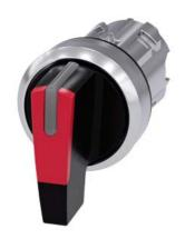
Selector switch, illuminable, 22 mm, round, metal, shiny, red, selector switch, long, 3 switch positions I-O-II, latching, actuating angle 2x45°, 10:30h/12h/13:30h, Z=50-unit packaging
