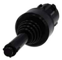
Coordinate switch, 22 mm, round, plastic, black, 4 switch positions, latching, with mechanical interlocking, with laser labeling, lower case  $\frac{1}{2} \frac{1}{2} \frac{1}{2}$
