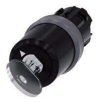
Key-operated switch BKS, 22 mm, round, plastic with metal front ring, lock number S1, with 2 keys, 2 switch positions O-I, latching, actuating angle  $90^\circ,$  10:30h/13:30h, key removal O+I, with laser labeling, upper case and lower case, always upper case at beginning of line
