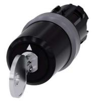
key-operated switch Siemens, 22 mm, round, plastic with metal front ring, lock number SSG10, with 2 keys, 3 switch positions I-O-II, latching, actuating angle 2x45°, 10:30h/12h/13:30h, key removal I, with laser labeling, upper case and lower case, always upper case at the beginning of the word
