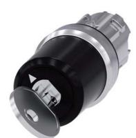
key-operated switch Siemens, 22 mm, round, metal, shiny, lock no. STGH10, with 2 keys, 2 switch positions O<I, momentary contact type, actuating angle 45°, 10:30h/12h, key removal O, with laser labeling, inscription or symbol customer-specific selection with SIRIUS ACT configurator (CIN)
