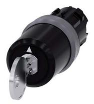
key-operated switch Siemens, 22 mm, round, plastic with metal front ring, special lock, with 2 keys, 3 switch positions I-O-II, latching, actuating angle 2x45°, 10:30h/12h/13:30h, key removal II
