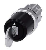
Key-operated switch BKS, 22 mm, round, metal, shiny, special lock, with 2 keys, 3 switch positions I-O-II, latching, actuating angle 2x45°, 10:30h/12h/13:30h, key removal O, Note: BKS locking systems E1 - E25 supplied without key
