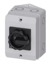
SENTRON, Switch disconnector 3LD, main switch, 3-pole, lu: 32 A, Operating power / at AC-23 A at 400 V: 11.5 kW, molded-plastic encapsulation for inch cable gland, 1 NC, 3 NO, rotary operating mechanism, black
