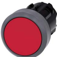
Pushbutton, 22 mm, round, plastic with metal front ring, red, pushbutton, flat momentary contact type, with laser labeling, upper case and lower case, always upper case at the beginning of the word
