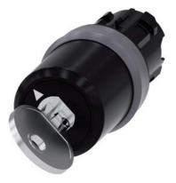
key-operated switch Siemens, 22 mm, round, plastic with metal front ring, lock number SSG10, with 2 keys, 2 switch positions O-I, latching, actuating angle  $90^\circ, 10:30\text{h}/13:30\text{h}$ , key removal O+I, with laser labeling, upper case and lower case, always upper case at beginning of line
