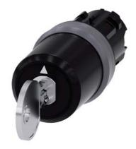
key-operated switch Siemens, 22 mm, round, plastic with metal front ring, lock number SSG10, with 2 keys, 3 switch positions I-O<II, left latching, momentary contact type on the right, actuating angle  $2x45^{\circ}$ , 10:30h/12h/13:30h, key removal I, with laser labeling, lower case
