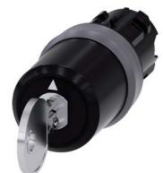
key-operated switch Siemens, 22 mm, round, plastic with metal front ring, lock number SSG10, with 2 keys, 3 switch positions I-O<II, left latching, momentary contact type on the right, actuating angle  $2x45^{\circ}$ , 10:30h/12h/13:30h, key removal O+I Z=50-unit packaging
