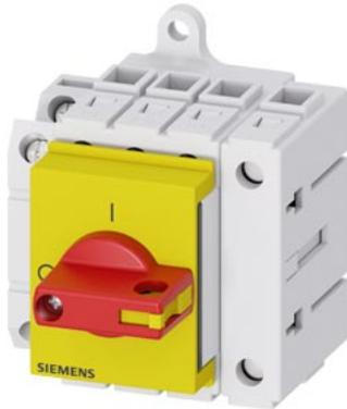
Load disconnecter 3LD3, Iu 63 A Main switch 3-pole + N Rated operating capacity at AC-23 A at 400V 22.0 kW Installation in distribution boards, Basic switch with selector knob red / yellow with auxiliary switch 1OE + 1S
