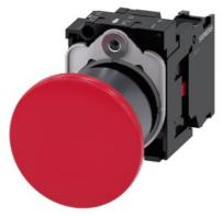
Mushroom pushbutton, 22 mm, round, plastic with metal front ring, red, 40mm, latching, pull-to-unlatch mechanism, with holder, 1 NC, screw terminal, with laser labeling, inscription or symbol Customer-specific selection with SIRIUS ACT configurator (CIN)
