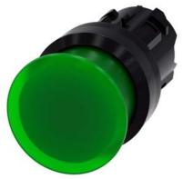
Illuminated mushroom pushbutton, 22 mm, round, plastic, green, 30 mm, momentary contact type, with laser labeling, upper case
