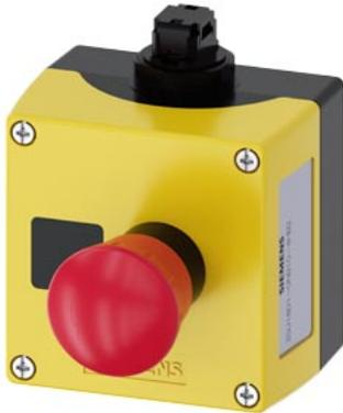
AS-Interface enclosure for command devices, 22 mm, round, Enclosure material plastic, Enclosure top part yellow, 1 control point plastic, Recess for label, A=EMERGENCY STOP mushroom pushbutton red, 40 mm, rotate-to-unlatch, 1 NC, 1 NC, spring-type terminal, floor mounting, Insulation displacement system on top, Label enclosed
