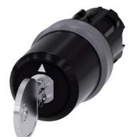
Key-operated switch BKS, 22 mm, round, plastic with metal front ring, lock number S1, with 2 keys, 3 switch positions I-O-II, latching, actuating angle 2x45°, 10:30h/12h/13:30h, key removal I, with laser labeling, upper case and lower case, always upper case at beginning of line
