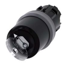
Key-operated switch IKON, 22 mm, round, plastic with metal front ring, lock number 360012K1, with 2 keys, 2 switch positions O-I, latching, actuating angle 90°, 10:30h/13:30h, key removal O+I, with laser labeling, upper case
