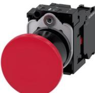
Mushroom pushbutton, 22 mm, round, plastic, red, 40mm, latching, pull-to-unlatch mechanism, with holder, 1 NC, screw terminal, with laser labeling, symbol number according to, ISO 7000 or IEC 60417
