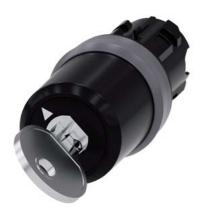
key-operated switch Siemens, 22 mm, round, plastic with metal front ring, lock number SSG10, with 2 keys, 2 switch positions O-I, latching, actuating angle 90°, 10:30h/13:30h, key removal O+I, with laser labeling, upper case and lower case, always upper case at the beginning of the word
