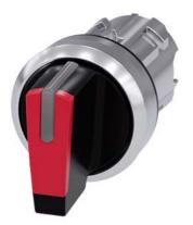
Selector switch, illuminable, 22 mm, round, metal, shiny, red, selector switch, short, 3 switch positions I>O<II, momentary contact type, actuating angle 2x45°, 10:30h/12h/13:30h, Z=50-unit packaging
