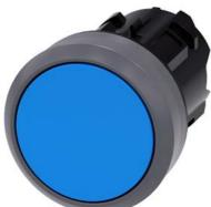
Pushbutton, 22 mm, round, plastic with metal front ring, blue, pushbutton, flat momentary contact type, with laser labeling, symbol number according to, ISO 7000 or IEC 60417
