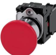
Mushroom pushbutton, 22 mm, round, metal, shiny, red, 40mm, latching, pull-to-unlatch mechanism, with holder, 1 NC, screw terminal, with laser labeling, upper case and lower case, always upper case at the beginning of the word
