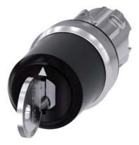
Key-operated switch IKON, 22 mm, round, metal, shiny, lock number 360012K1, with 2 keys, 3 switch positions I>O<II, momentary contact type, actuating angle 2x45°, 10:30h/12h/13:30h, key removal O, with laser labeling, inscription or symbol Customer-specific selection with SIRIUS ACT configurator (CIN)
