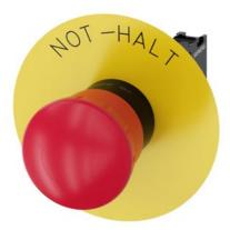
EMERGENCY STOP mushroom-type actuator, 22 mm, round, plastic, red, 40 mm, positive latching, according to EN ISO 13850, rotate-to-unlatch, with yellow backing plate, inscription: NOT-HALT, with holder, 1 NC, screw terminal, Z=20-unit packaging
