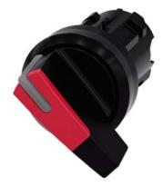
Selector switch, illuminable, 22 mm, round, plastic, red, selector switch, long, 2 switch positions O-I, latching, actuating angle  $90^\circ$ , 10:30h/13:30h, with laser labeling, lower case
