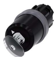
key-operated switch Siemens, 22 mm, round, plastic with metal front ring, lock no. LSG1, with 2 keys, 2 switch positions O-I, latching, actuating angle 90°, 10:30h/13:30h, key removal O, with laser labeling, upper case
