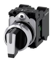
Selector switch, illuminable, 22 mm, round, metal, shiny, white, selector switch, short, 3 switch positions I>O<II, momentary contact type, actuating angle 2x45°, 10:30h/12h/13:30h, with holder, 1 NO, 1 NO, spring-type terminal, Z=20-unit packaging
