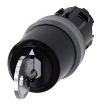
Key-operated switch IKON, 22 mm, round, plastic with metal front ring, lock number 360012K1, with 2 keys, 3 switch positions I-O-II, latching, actuating angle 2x45°, 10:30h/12h/13:30h, Key removal I+O+II, Z=50-unit packaging
