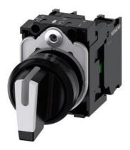
Selector switch, illuminable, 22 mm, round, plastic, white, selector switch, short, 3 switch positions I-O-II, latching, 10:30h/12h/13:30h, with holder, 1 NO, 1 NO, screw terminal, with laser labeling, upper case and lower case, always upper case at the beginning of the word
