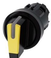
Selector switch, illuminable, 22 mm, round, plastic, yellow, selector switch, short, 3 switch positions I>O<II, momentary contact on the left, latching on the right, actuating angle  $2x45^{\circ}$ , 10:30h/12h/13:30h
